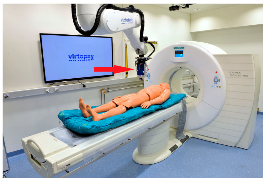
Figure 1. The Virtobot positioned above the CT gantry. The biopsy tool mounted to the robotic arm is located immediately above the dummy (red arrow).
