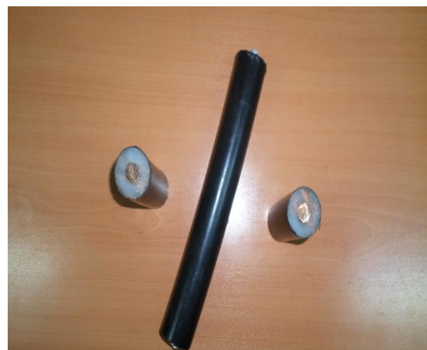
Fig. 1. XLPE insulated single core medium voltage cable
