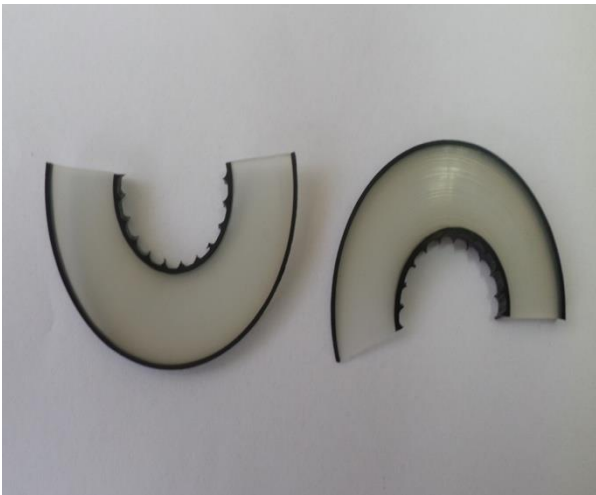
Fig. 2. Image of insulator sample taken from XLPE insulated single core medium voltage cable
