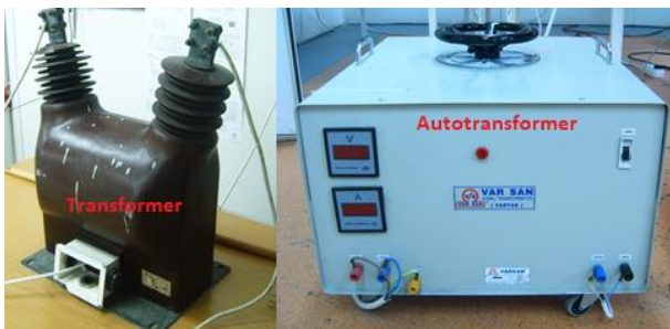
Fig. 1. The test transformer and autotransformer.
