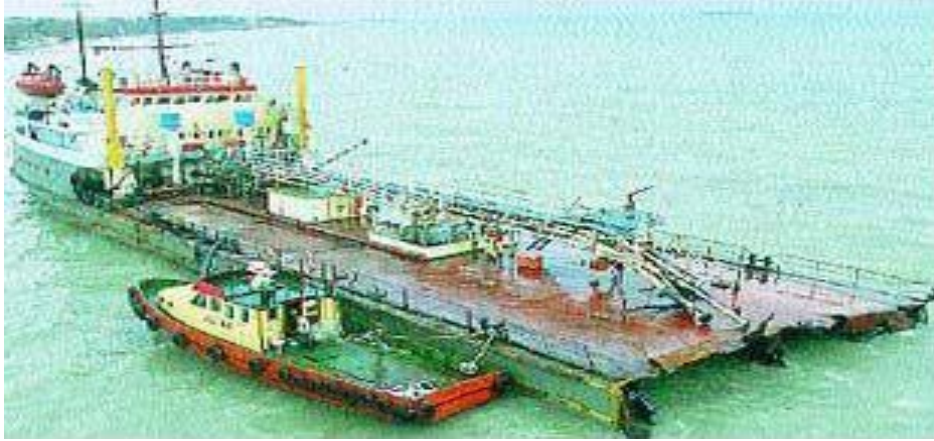
Figure 1. M/T VOLGONEFT 248 broke into two parts at an anchorage İstanbul in the Sea of Marmara. The bow section with four full tanks (No. 1-4) sank at 30 meters of waters with 2073 tons of oil.
