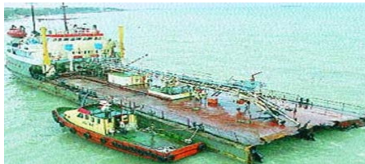
Figure 14. M/T Volganefit-248's stern part after the collision (from Turkish Straits Vessel Traffic Service).
