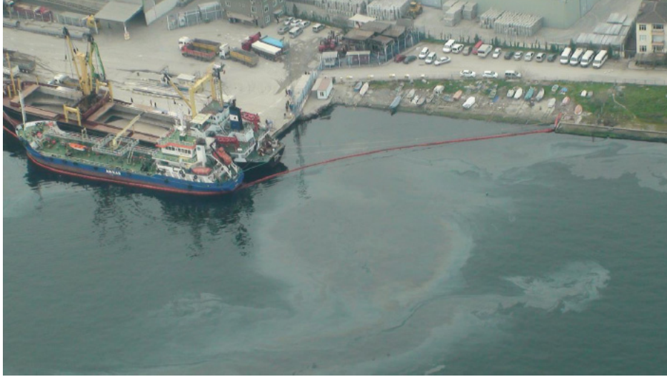
Figure 4. Polluting spreading outside the barrier (AMAL and URLA 1, KAİK Ship Accident Report)
