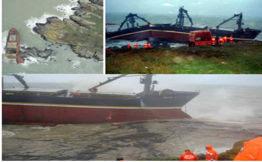
Figure 17. Rescue operations of the M/V Orçun-C which was broken into two parts ( http://www.denizhaber.com/deniz-kazalari/ ; Usluer, 2016).
