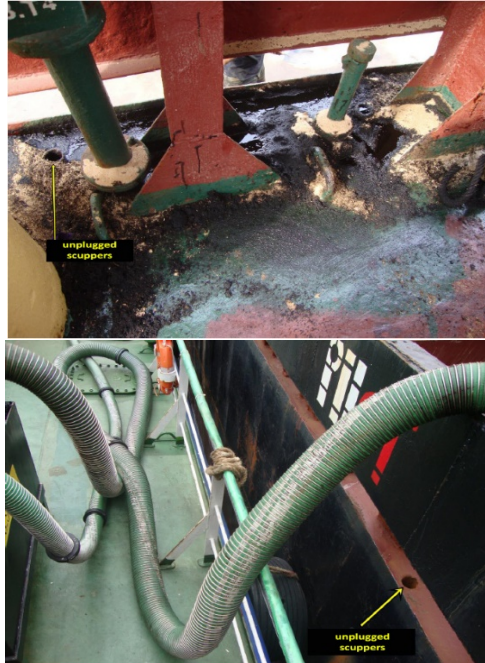
Figure 3. Unplugged scuppers on the vessel AMAL (AMAL and URLA 1, KAIK Ship Accident Report).
