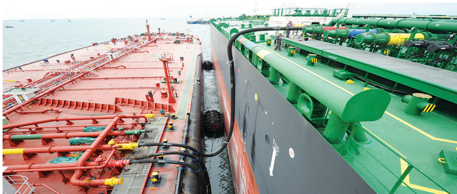
Figure 2. Bunkering operation (from marineinfobox.blogspot.com ).
