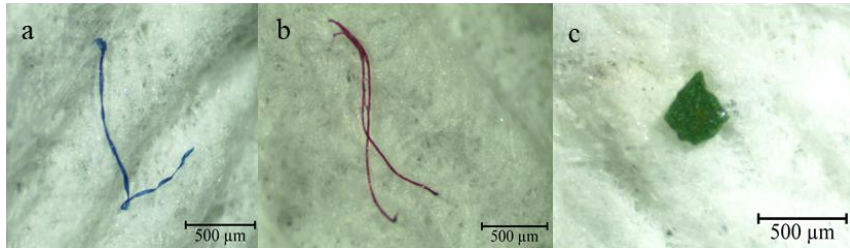
Figure 3. Examples of microplastic types found in bivalve species (a: film, b: fibre, c: fragment)
